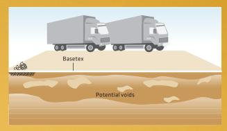
Basetex can provide safe, early warning of the development of voids below earthworks.
