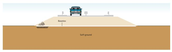
$Base tex\ is\ usually\ placed\ as\ low\ as\ possible\ within\ the\ embankment\ foundation\ to\ maximise\ stability.$
